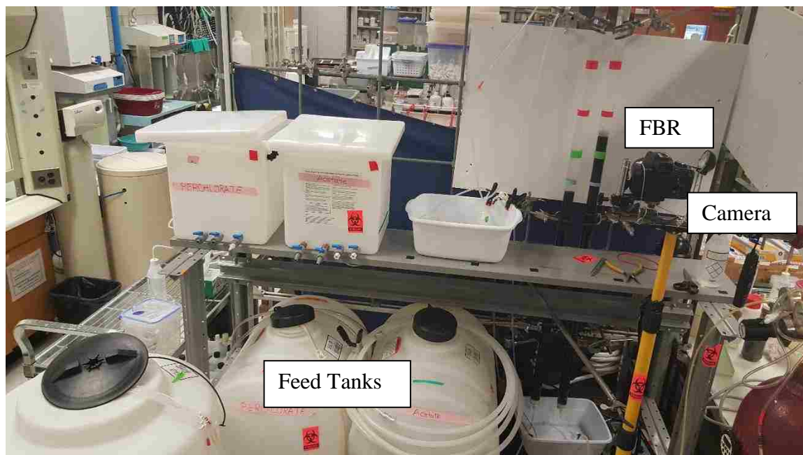
Figure 5.2: Experimental set up for operating two FBRs with camera mounted to take pictures.
